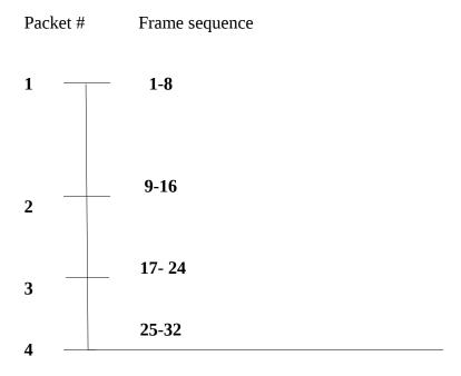
4 packets of 2048bytes burst with frame sequences of 8.
