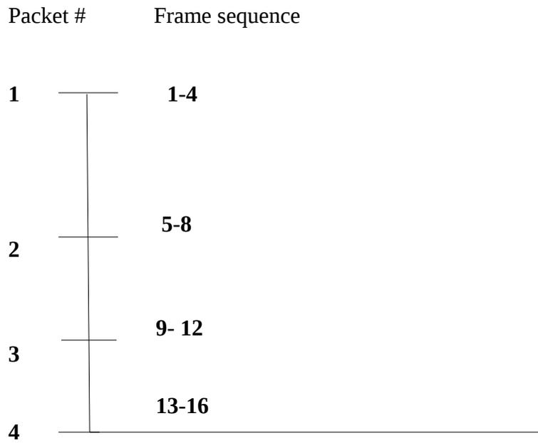
**4 packets of 3072bytes burst with frame sequences of 4.**
